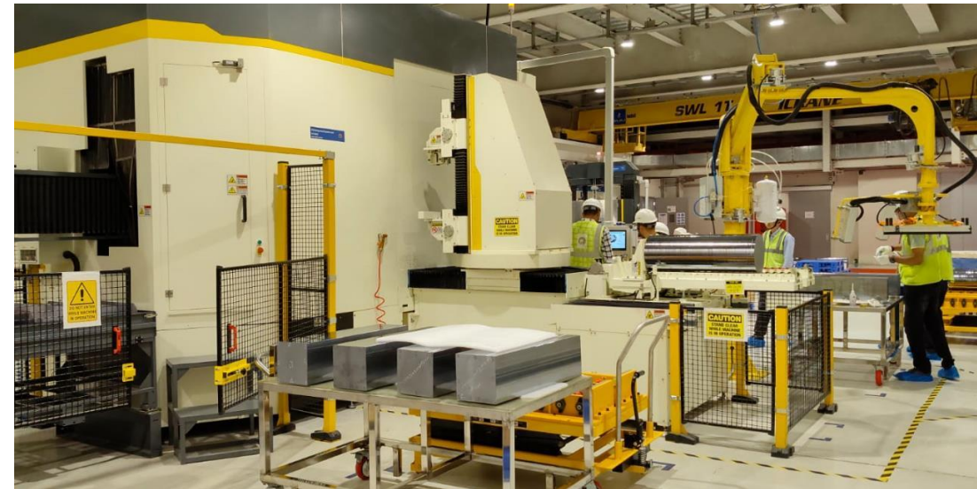
Ingots are cropped into 'bricks'
