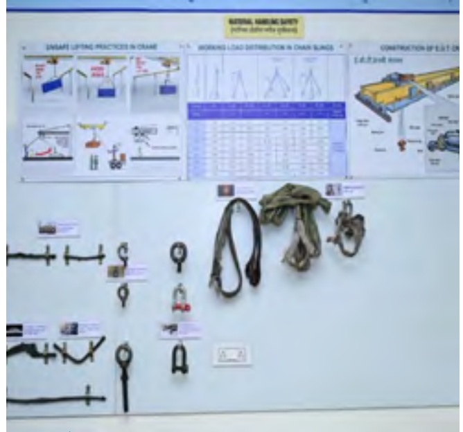
Forklift Safety, Crane Safety, Safe use of Lifting tools and tackles, Safety of Racking system with rack inspection information displayed
