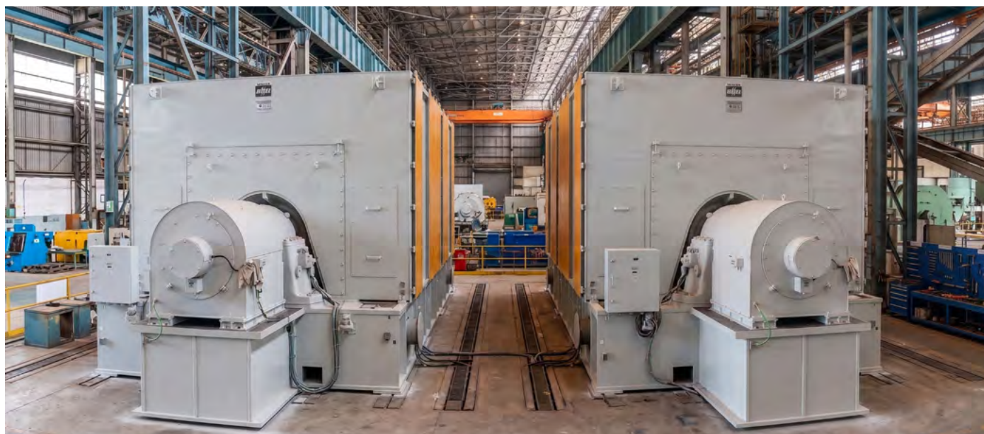
BHEL's highest-rated air-cooled Synchronous Generators - 4 nos 175 MW Generator manufactured for Jindal Mmamabula Energy Project, Botswana
