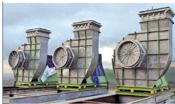
Process Exhaust Blowers for Solar Manufacturing Unit
